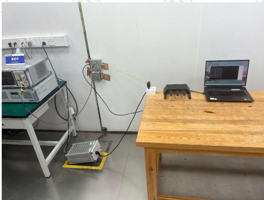
Conducted emissions Test Setup-1
