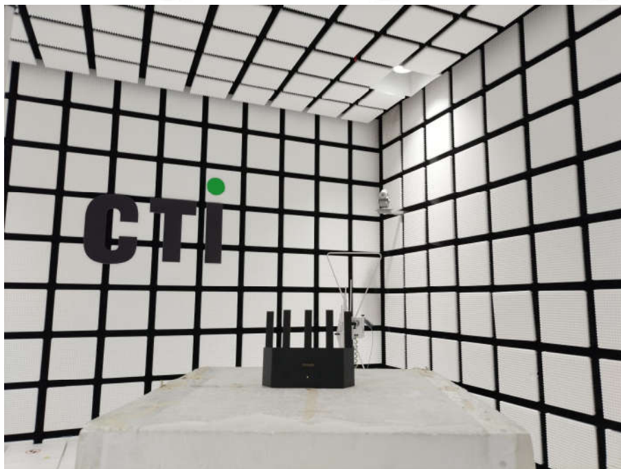
Radiated spurious emission Test Setup-1(Below 1GHz)
