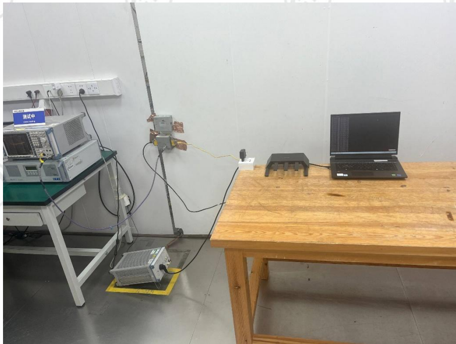
Conducted emissions Test Setup-2
