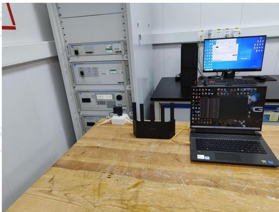
Voltage dips and interruptions Test Setup-2
