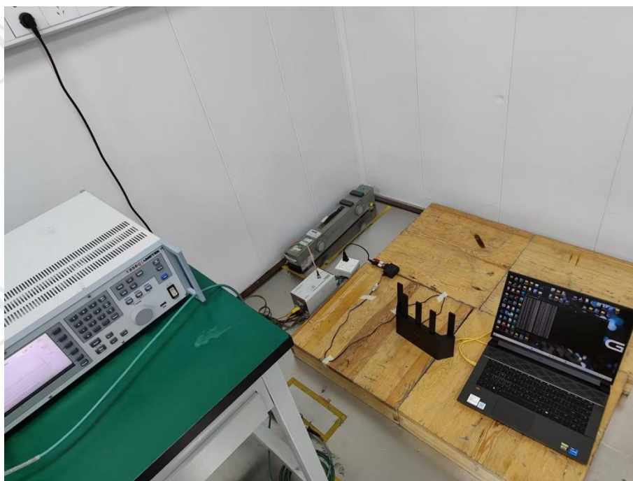
Continuous induced RF disturbances Test Setup-1
