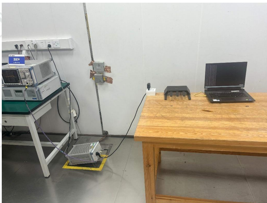
Conducted emissions Test Setup-3
