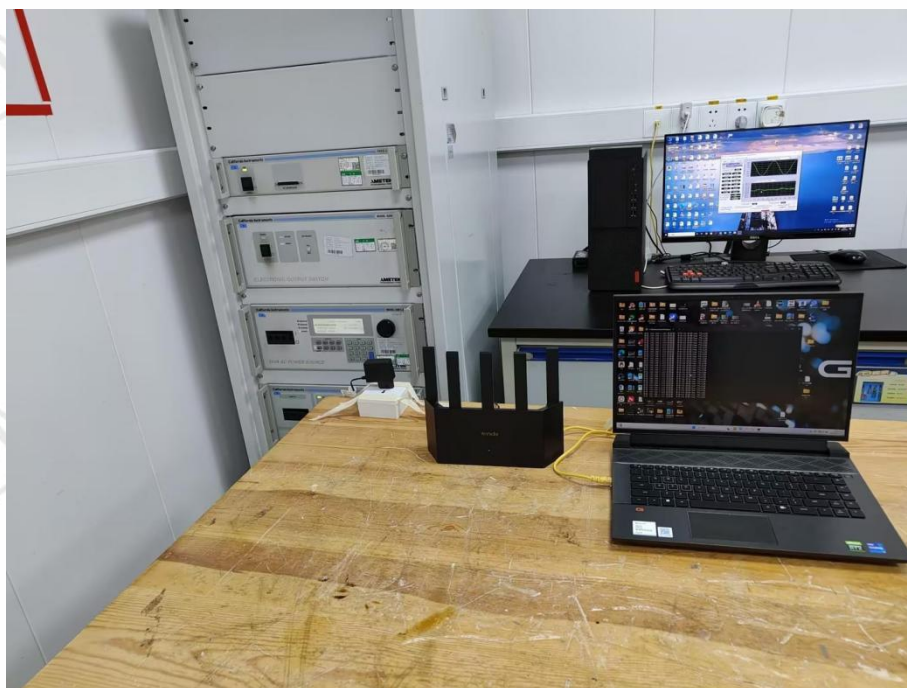
Voltage changes voltage fluctuations and flicker Test Setup-2
