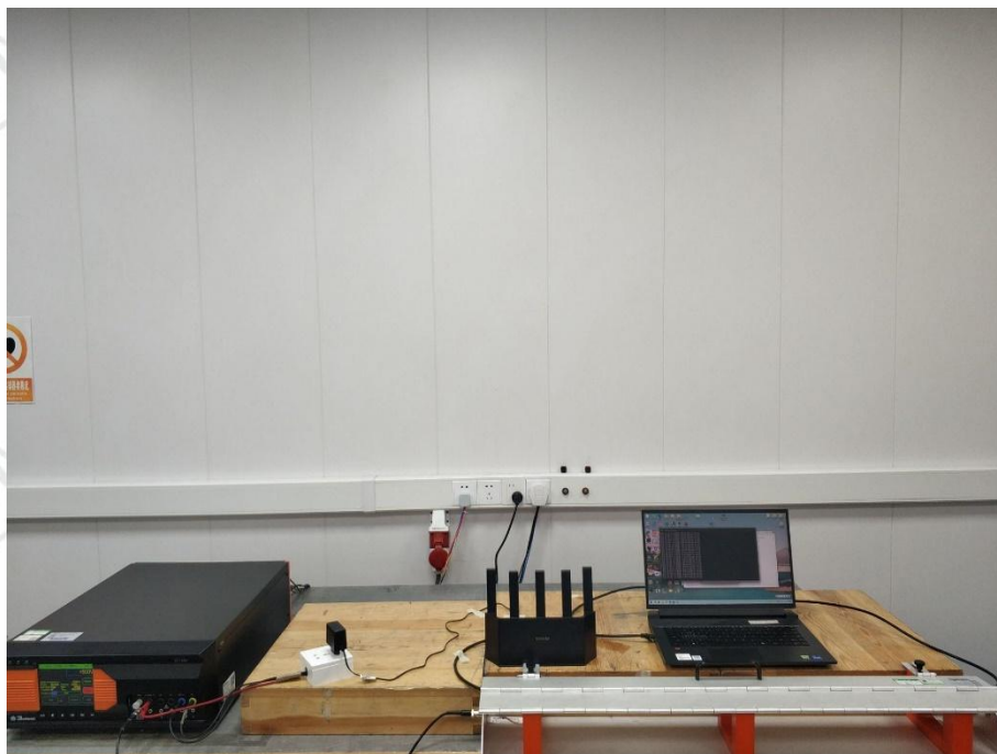
Electrical fast transients burst Test Setup-2
