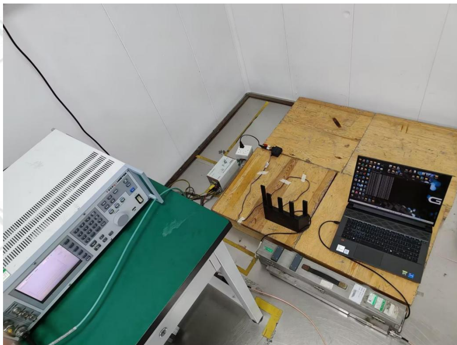
Continuous induced RF disturbances Test Setup-3
